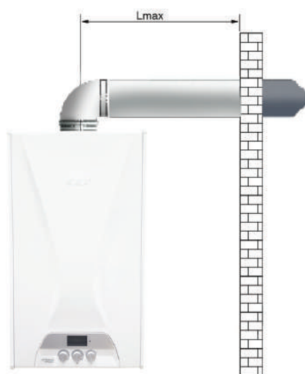
Horizontal Hermetic Flue Application (Lmax distance with one elbow: 4 m, Ø60/100) (Lmax distance with one elbow: 6 m, Ø80/125)
